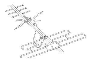
Step 8 Attach U bolt and mast clamp as per diagram.
