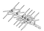
Then attach corner reflector using the two screws and wing nuts provided as per diagram.
