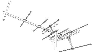
2) Snap out front and back corner reflectors located on the back 778mm boom.
