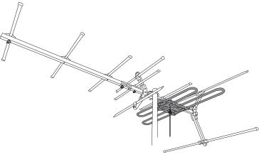
4) Join the front 684mm boom to the back 778mm boom using the 3/16" Philips/flathead bolt, spring washer and wingnut provided in the small plastic bag. Make sure you install the spring washer and wingnut on the underbody of the boom body.
