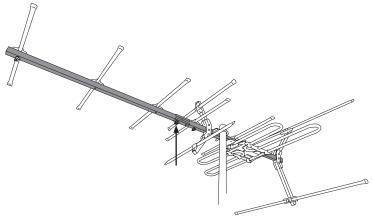
5) Install the two 520mm swivel lock elements included to the top of the booms using the pre-drilled holes located at the front and middle of the joining booms.
