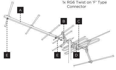
1) Snap out two riveted swivel lock elements located on the front 684mm boom and five riveted swivel lock elements situated on the back 778mm boom.
