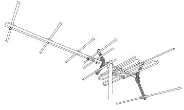
3) Attach the G-unit to the back 778mm boom underbody, lining up the pre-drilled holes located on the G-unit and boom. Bolt these two units together using the 1/4" bolt, flat washer, spring washer and wingnut provided in the small plastic bag. Make sure you install the flat washer, spring washer and wingnut on top of the boom body.
