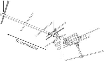
6) Attach the antenna to the mast using the U-bolt and point to your nearest transmitter. Slide the rubber boot seal into your coaxial cable. Strip the coaxial cable and attach the connector provided, then connect to the antennas balun. Fix the coaxial cable down the mast using UV grade insulation tape and cable ties.
