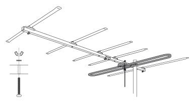
2) Attach the dipole to the back 558mm boom underbody, lining up the pre-drilled holes located on the dipole and boom. Please ensure dipole is installed with balun towards the front of the antenna. Bolt these two units together using the M5 bolt, star washer, and wingnut provided in the small plastic bag. Ensure you install the star washer and wingnut on top of the boom body.
