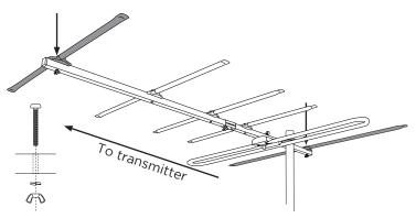
4) Install the front 532mm swivel lock element to the front 630mm boom located at the front and 900mm swivel lock element to the top of the back 558mm boom using the pre-drilled hole situated at the back.
