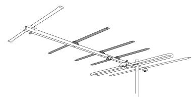
1) Snap out the two riveted swivel lock elements on the front 630mm boom and one on the back 558mm boom.
