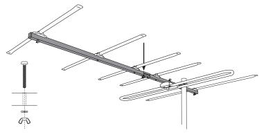
3) Rotate the front and back booms, so the riveted swivel lock elements are on top of the front and back boom. Join the front 630mm boom to the back 558mm boom using the 3/16" Philips head screw, spring washer and wingnut provided in the small plastic bag. Make sure you install the spring washer and wingnut on the underbody of the boom body.
