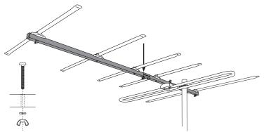
3) Rotate the front and back booms, so the riveted swivel lock elements are on top of the front and back boom. Join the front 630mm boom to the back 558mm boom using the 3/16" Philips head screw, spring washer and wingnut provided in the small plastic bag. Make sure you install the spring washer and wingnut on the underbody of the boom body.
