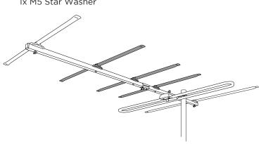
1) Snap out the two riveted swivel lock elements on the front 630mm boom and one on the back 558mm boom.
