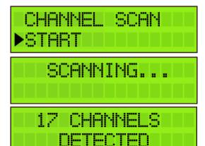
Scroll down to START and tap the rotary button to start scanning
