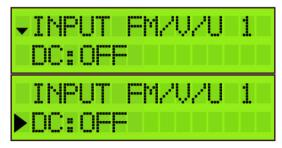
Rotate the rotary button to scroll down in the submenu.
