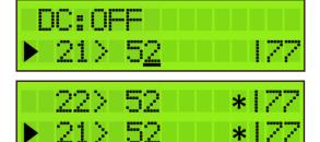
Example of adding a channel with Channel conversion active.
