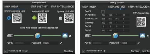
Please follow the prompts of the startup Wizard to install the CCTV system after connecting power and switching on.
