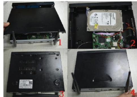
1. Remove the screws as indicated in diagram above and remove the cover
