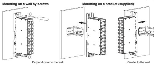
Figure 1. Mounting of the splitter
